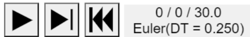
Figure 7.1. The execution buttons: Run/Pause , Step and Reset . (To the right of the buttons the Start Time / Actual simulation time / End Time (before the run) and below the Method and Time Step are displayed).
