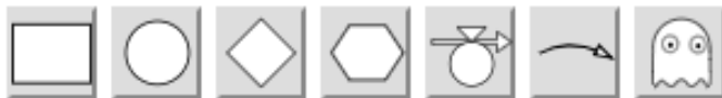
Figure 4.1. The buttons for StochSD building blocks: Stock , Auxiliary , Parameter , Converter , Flow , Link and Ghost .
