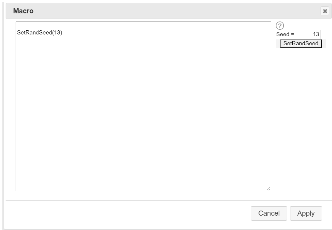
Figure 11.1. In the Macro form, you can define a macro function of your choice. It can also be used to make a stochastic simulation reproducible by selecting a Seed (a number that initiate the random number generators) and click the button SetRandSeed .
